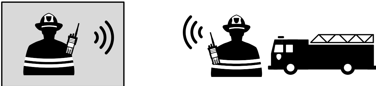
With Fire Ground Simplex communications, the radio inside the building will talk directly with a radio outside the building. No Radio Infrastructure is involved. This radio channel is Channel 16 on your Primary Zone and it is a Digital 700 MHz frequency.
