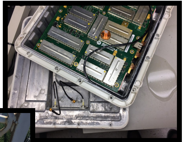
Above: Water damaged outdoor microwave equipment from the 'Maxwell Hill' radio site. Radio Systems had a significant increase in storm related and other damage to system infrastructure. Redundant systems and prioritized repair procedures kept all systems functioning throughout the year regardless of individual subsystem failures.
